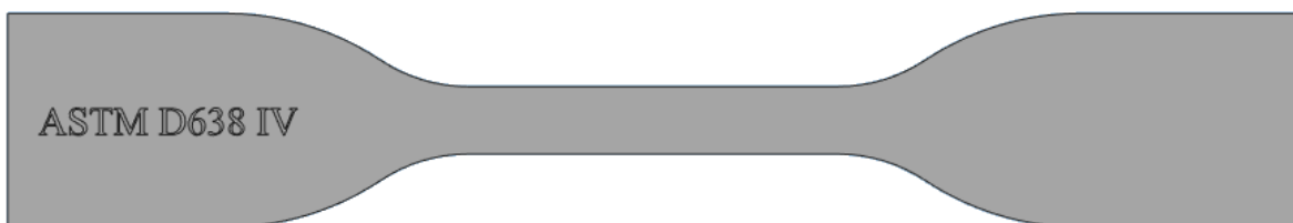
Figure 1 Tensile bar ASTM D638 IV
